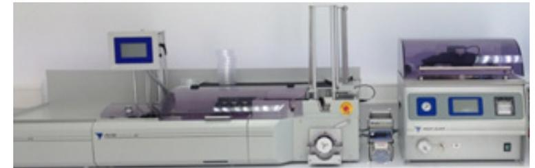
high throughput setup with blood addition pump and ProfiClave Agar preparator
